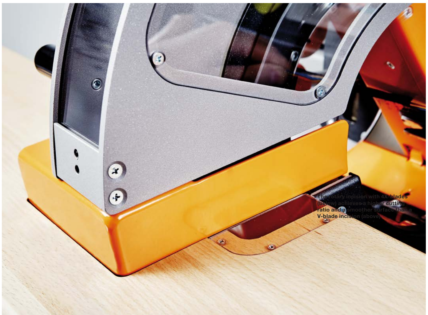
01 The tape end detection sensor (optionally available) ensures optimum production processes.
